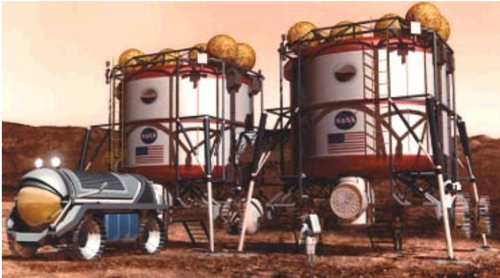
FIGURE 8. Class 1, Pre-integrated “Tuna Can” hard module, landed complete on the lunar or Mars surface. Credit: John Frassinito and Associates, circa 1993.
