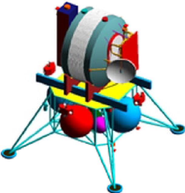
Figure 7a. Lunar Return Habitat in landing position with the inflatable habitat and equipment stowed. Credit Kriss Kennedy, NASA-JSC.
