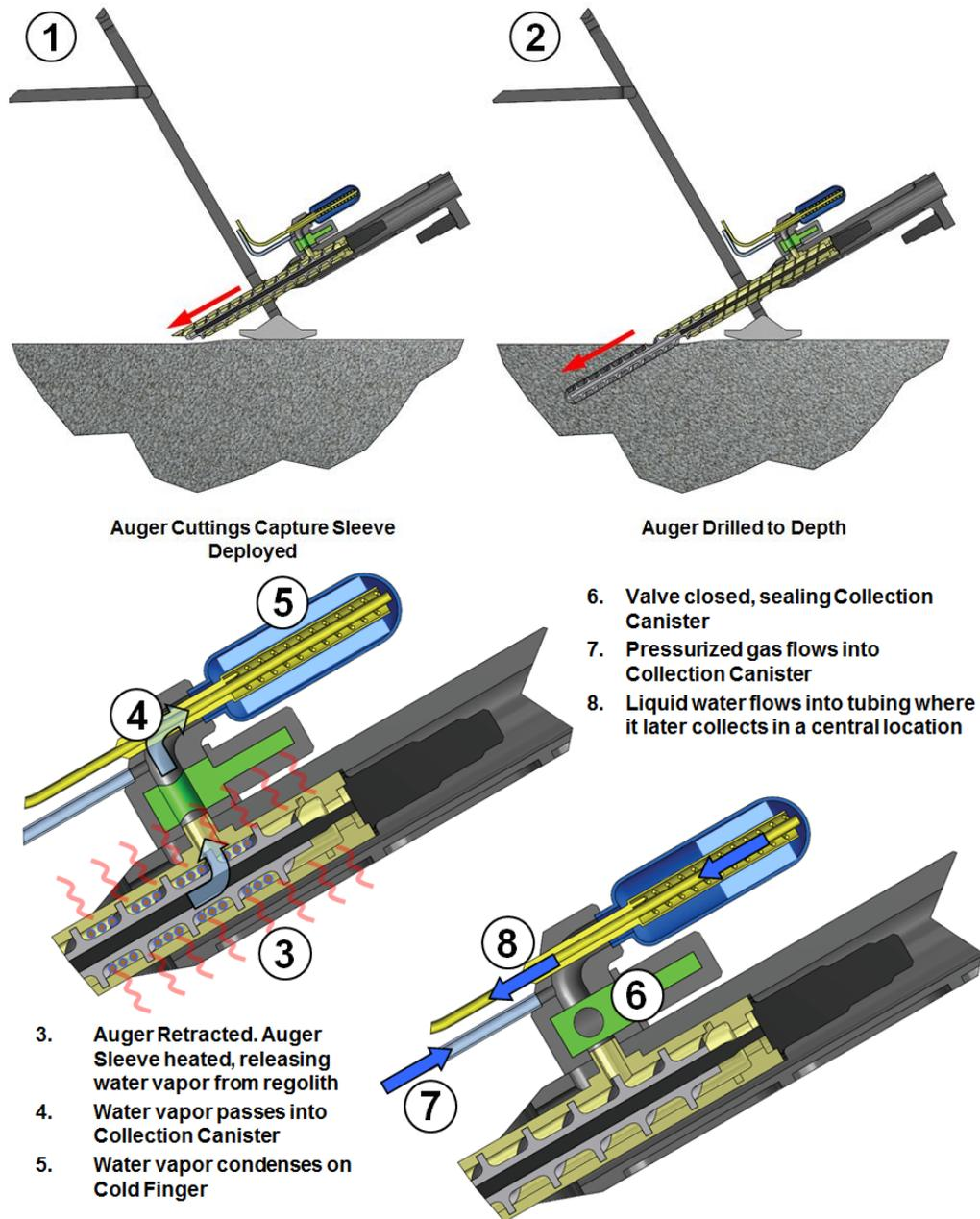
**Figure 9. Water Extraction and Condensation Process**
