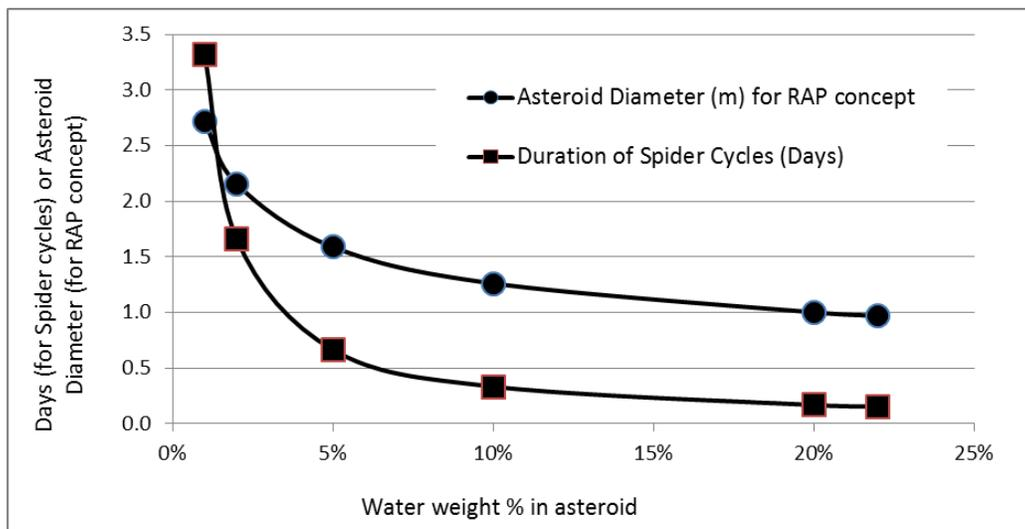
**Figure 10. Diameter of an asteroid for the RAP spacecraft or duration of Spider cycles required to recover 100 kg of water as a function of water wt% in asteroid regolith. Water extraction efficiency assumed at 50% in both cases.**
