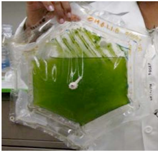
FIGURE 7. Experimental Green Algae Growth FO Bag (Trent et al, 2010).
