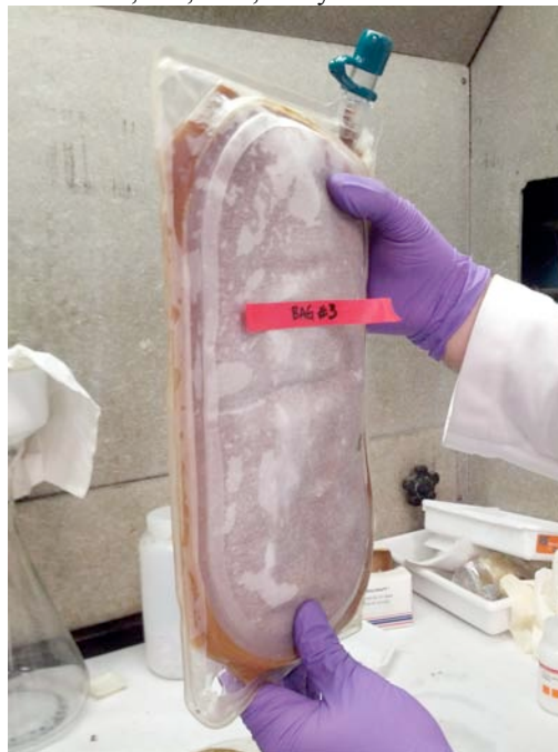
FIGURE 1. Fecal Simulant Bags for Radiation Beam Testing. Simulant prepared by Jurek Parodi, Serena Trieu, and Kevin Howard, University Space Research Association at Ames Research Center.
